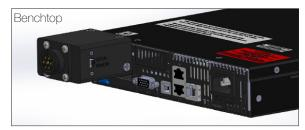
Benchtop Option: Unit attached to the back of the standard LPS-400 or 850 that converts from terminal outputs to our standard HIS or HES cable adapter. Fan power inputs (from wall wort) and a selector switch that enable the fan power are included. Also includes wall power supply with radio jack for 30W/12V/2.5A power to the fan (Part#1035-2). The wall power supply is required for the HES lamps (integral fan) but not for the HIS lamps.
